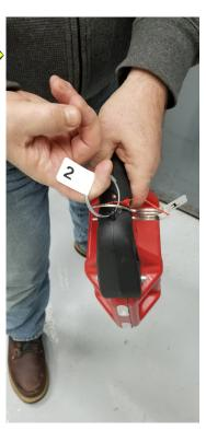
Pulling the pins in the incorrect order will cause the SUPPRESSALL FS2 to fail. It will not deploy.
